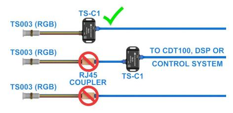
The TS-C1 requires an extra wire to connect to the General-Purpose output or relay block to light up
